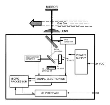
Figure 5-2 Block diagram, GD10PE
