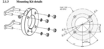
Figure 2-5 Exploded view, Duct Mount Flange Kit with recommended installation boredimensions.
