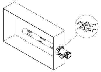
Figure 2-1 One-sided duct mounting using Mounting Flange Kit.
