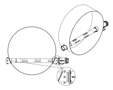
Figure 2-3 Circular duct mounting using Guide Support Kits and Extension Kit.
