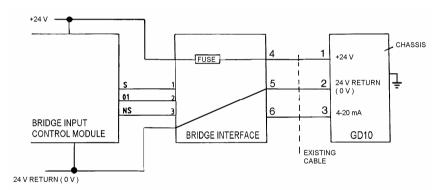
Figure 2-8 Bridge interface installation
