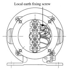
Terminal 1 +24 V DC Terminal 2 24 V return (0 V) Terminal 3 4-20 mA output
