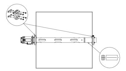
*Figure 2-2 Dual side duct mounting using two Flange Mounting Kits and Extension Kit*
