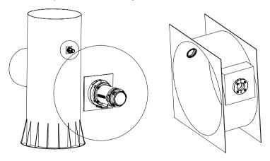
Figure 2-4 Mounting Flange Kit used on circular duct segments.
