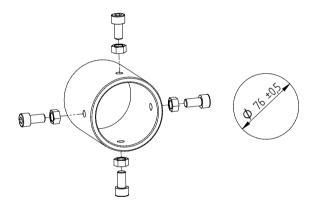
Figure 2-6 Exploded view, Guide Support Kit, with recommended installation bore dimension. Welding required.
